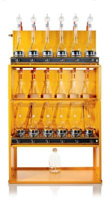
Combined apparatus for classic, manual nitrogen determination using the Kjeldahl method. The space-saving alternative to two individual pieces of equipment. Sturdy design in tried and tested C. Gerhardt quality. For 6 digestion and 6 distillation processes simultaneously.
