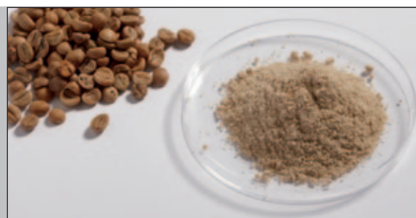
Raw coffee before and after grinding with the P-14 and sieve ring 1 mm trapezoidal perforation at 20,000 rpm
