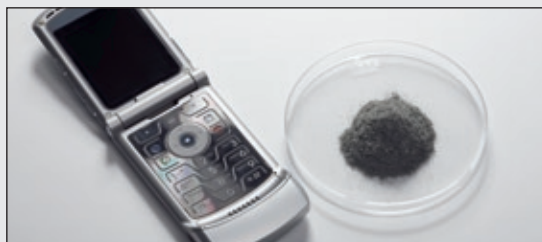
Mobile phone keypad: Grinding results after embrittlement under freezing conditions
