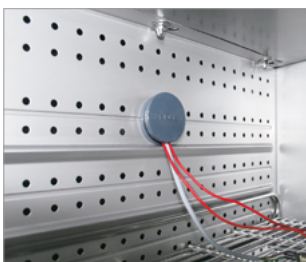
Access port with silicone plug
