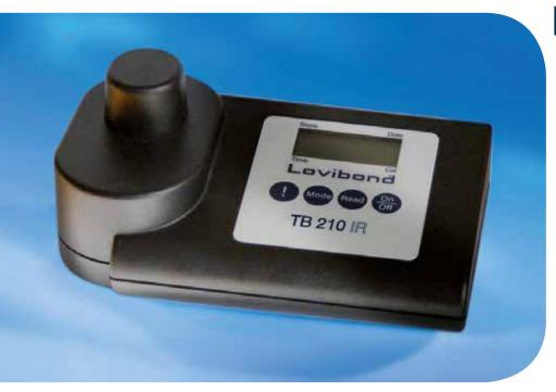
The compact Lovibond® infrared turbidity meter TB 210 IR is designed to allow fast, precise on-site testing. The unit measures the scattered light at an angle of 90°, as stipulated in EN ISO 7027.
