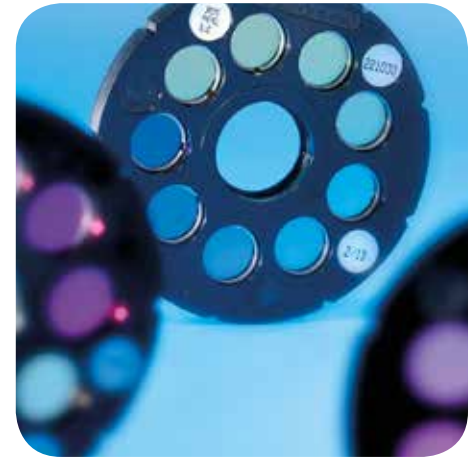
Test disc with colour-stable glass standards
